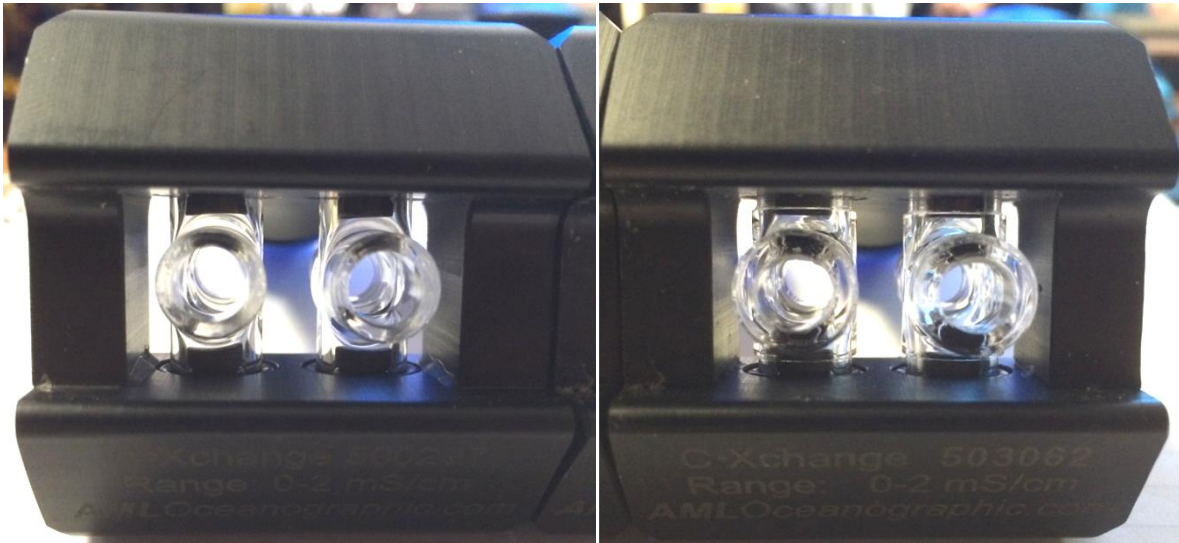
Left: Borosilicate glass cross tubes. Right: Fused quartz glass cross tubes. Note the thicker glass tubes on the right (fused quartz) sensor.
