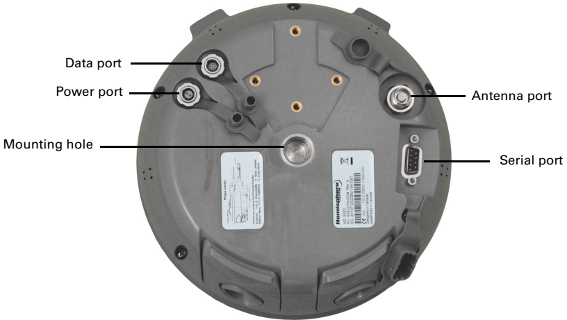
Figure 2-1: S320 ports and connectors
