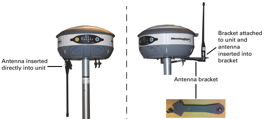
Figure 2-2: Antenna installation options
