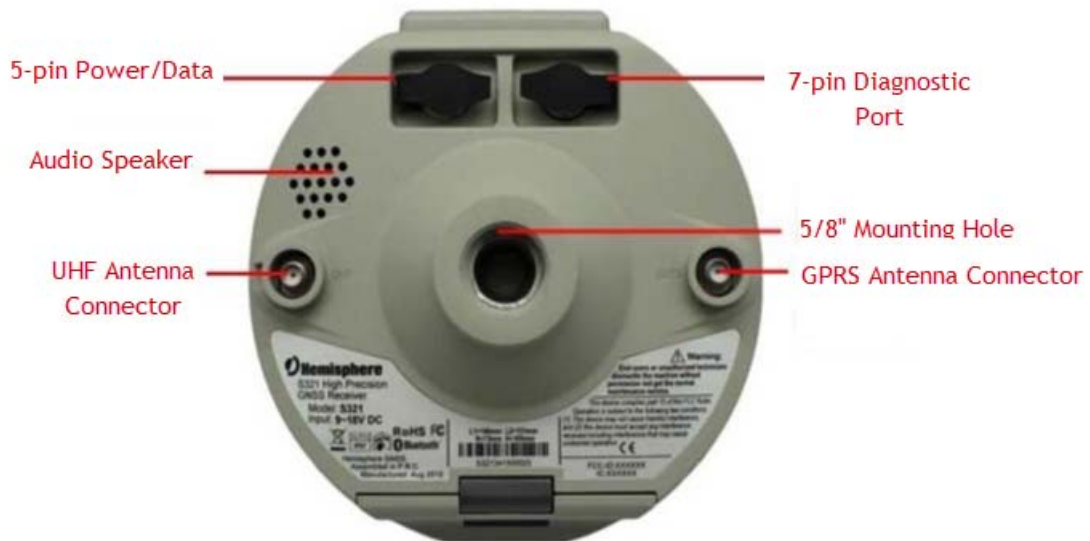
Figure 2-1: S321 ports and connectors
