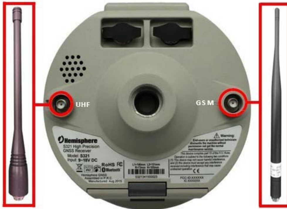
Figure 2-3: Installing UHF and GSM antennas
