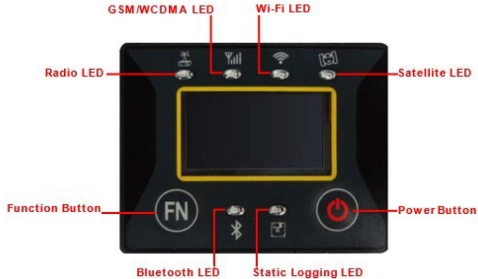
Figure 3-1: Control panel and display
