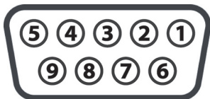
Figure 3-8: DB9 female socket numbering
