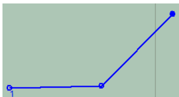
FIGURE 71. Survey Line Extended 45 Survey Units at a Bearing of 45 Degrees
