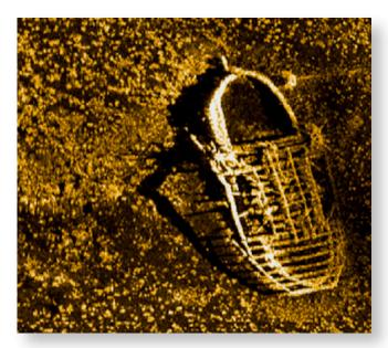
In the image above: The Burlington Horse Ferry, in Lake Champlain, VT. Image taken with Klein 4900 at 900Khz, 60m swath, 4knots, captured on the port side. Software: Klein SonarPro®.
