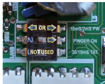
FIGURE 9 Switch SW1 positions for pinger operation
