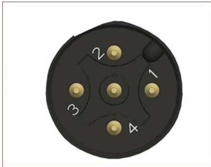
Figure 2-10: 5-pin (male) CAN port pin-out
