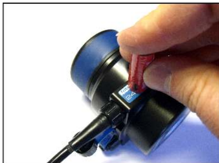
Figure 5.1. Location of Reset Switch (activated by magnet)
