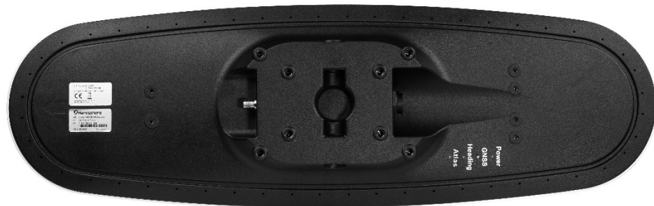
Figure 2-5: Flush-mounting holes on bottom of V500
