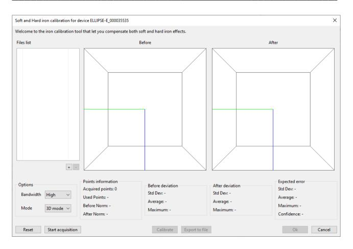
Bandwidth should be left on High and the Mode where possible set to 3D when ready click the start acquisition button to start the magnetometer readings.
