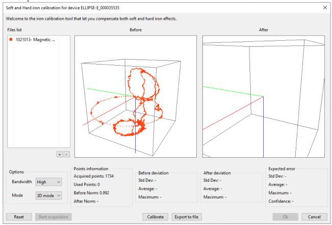
Check that the 3D method is used (in case of very large ship, or when the roll/pitch angles could not be changed significantly during calibration, a 2D method can be used). Press "Calibrate" and check calibration results.
