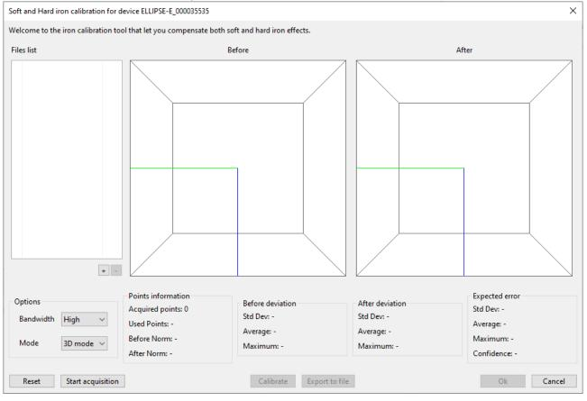
Bandwidth should be left on High and the Mode where possible set to 3D when ready click the start acquisition button to start the magnetometer readings.
