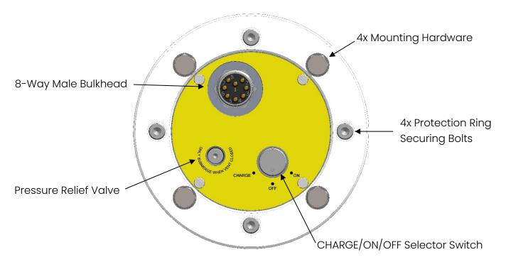
The Pressure relief value will automatically purge if a build-up of gases occurs inside the MiniPod, the PRV should be exercised regularly, such as after charging and greased if required to ensure continued safe operation see section 6.
