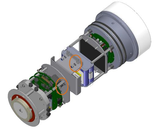
It is recommended that the battery pack is replaced every 3 years which is indicated on a battery expiry label fitted inside the endcap protection ring.
